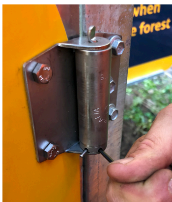
To adjust the gate strength, put a small pin or screwdriver & turn it to your right.
