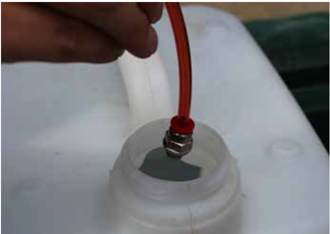
Insert the red hose into the sterigene tank first.
