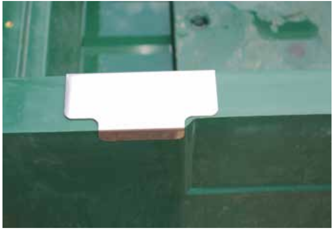
The back left mirror should align with the exterior moulded indents in the base as shown.
