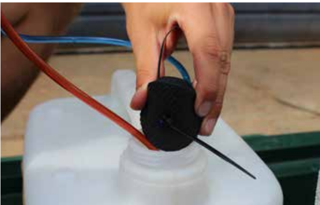
Then squeeze the foam floatie on the end of the blue hose and insert it into the sterigene tank.
