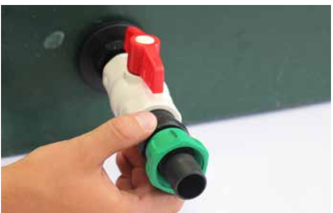
Screw it into the tank tap.
