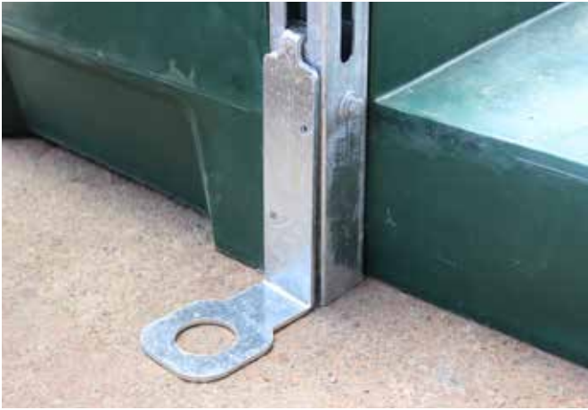
Rotate the bracket down until flush with the ground and vertical edges are in line with the upright.
