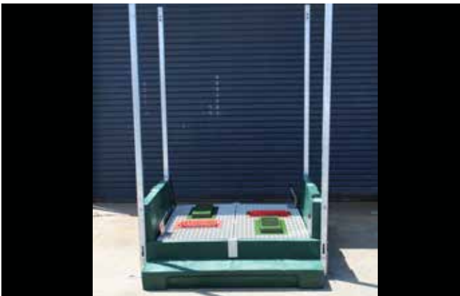
Repeat steps for installing uprights and earth anchor brackets onto each corner of the base as shown.
