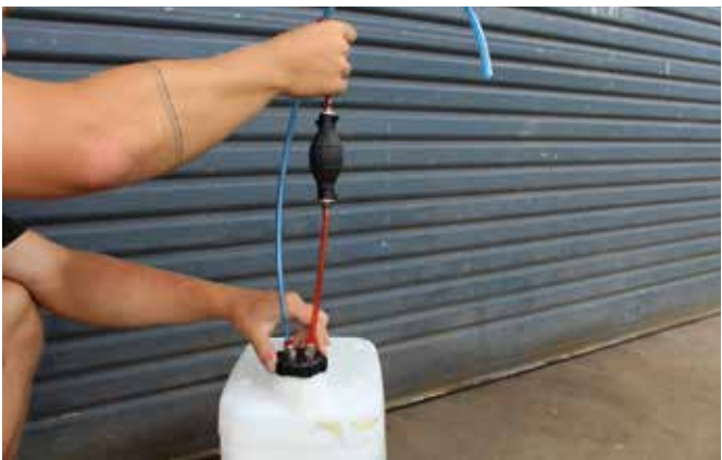
Screw the tank cap onto the sterigene tank tightly so it will not leak.
