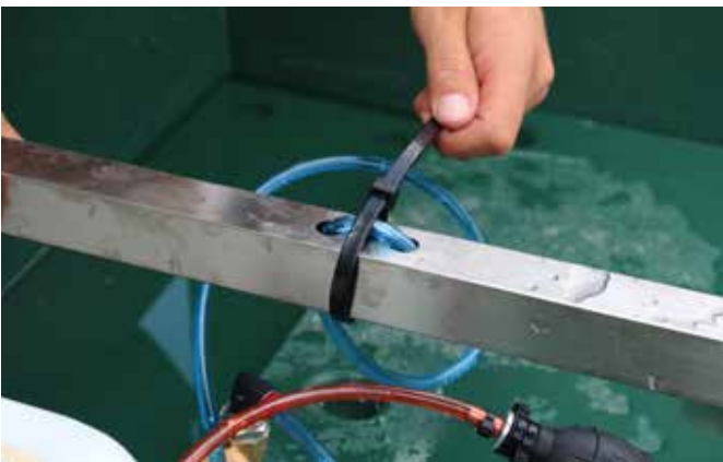
Tighten the adjustable cable tie, being careful not to squash the hose. Pull the locking mechanism of the cable tie underneath the middle support bar so it will not be in the way of the mesh.
