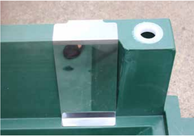
The front right mirror should sit hard against the internal corner of the base as shown, next to the plumbing thread.
