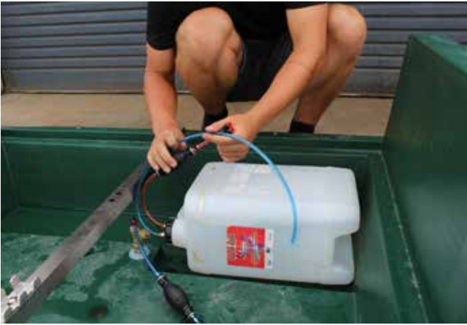
Ensure the sterigene tank is rectangular like shown, NOT square as this will not fit under the mesh.
