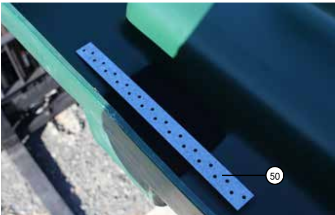
Lay the bracing strap over the foam centrally like so.
