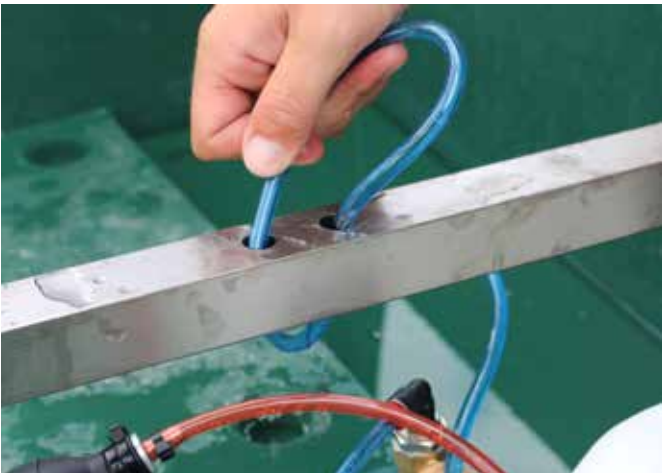
Loop it over and insert it into the next hole, pushing the hose along inside the middle support.
