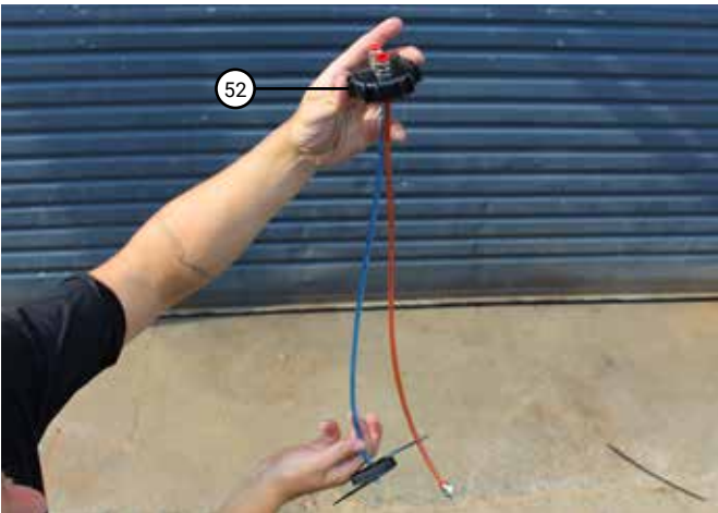
Take the tank cap assembly and ensure the floatie cannot pull off the blue hose and that the hoses are plugged into the cap securely.
