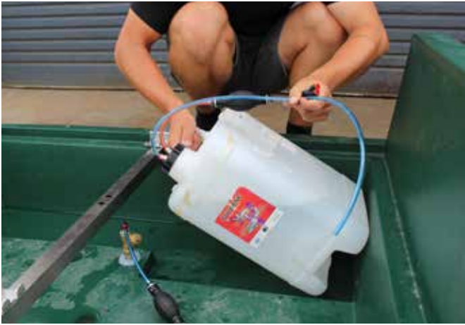
Lie the sterigene tank on its side in the bottom of the base in the rectangular divot with the cap next to the central plumbing assembly.
