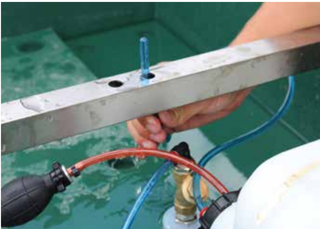
Lie the sterigene tank on its side in the bottom of the base in the rectangular divot with the cap next to the central plumbing assembly.
